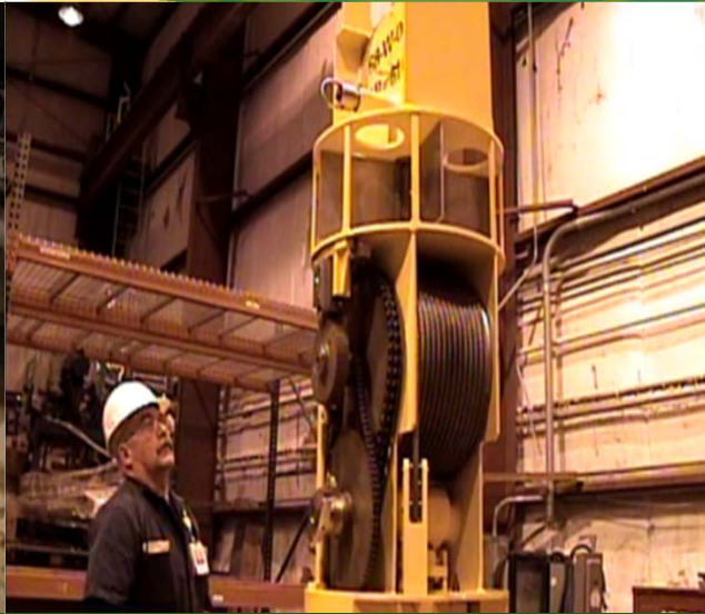
Testing Load Lowering Device
